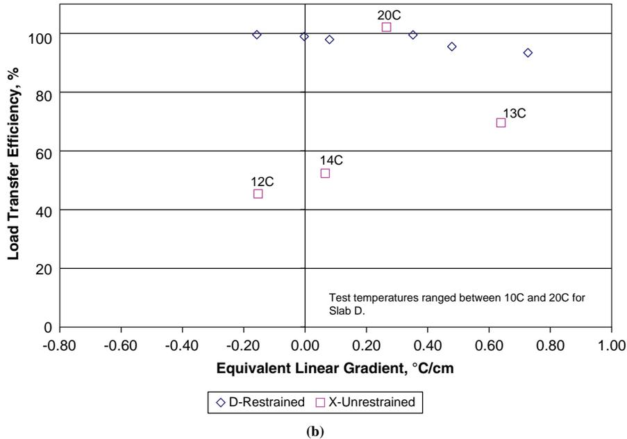
FIGURE 3 Relationship between load transfer and gradients for 190-mm (7.5-in.) slabs on asphalt-stabilized base: (a) Cell 7, slab length = 6.1 m (21 ft), and (b) Cell 8, slab length = 4.6 m (15 ft).
