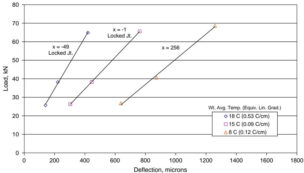
FIGURE 7 Deflections and loads measured in April for unrestrained slab in Cell 5.
