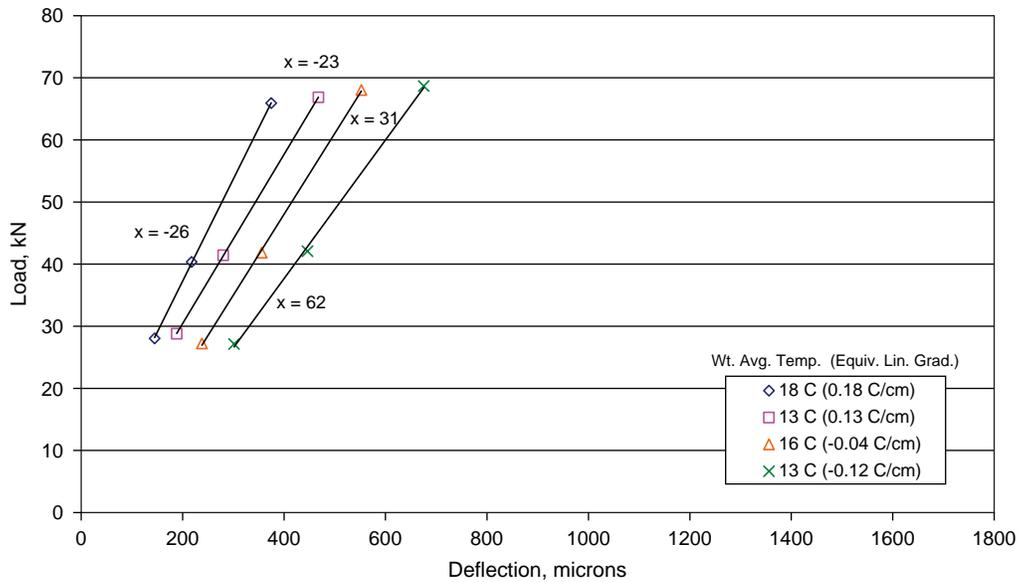
FIGURE 6 Deflections and loads measured in September for unrestrained slab in Cell 5.
