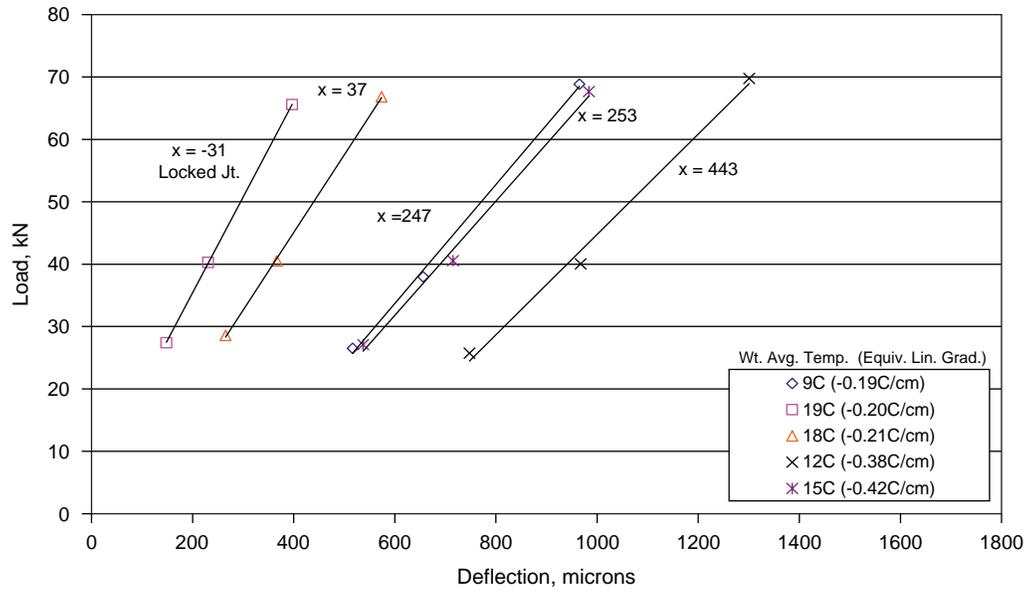
FIGURE 8 Deflections and loads measured in October for unrestrained slab in Cell 5.
