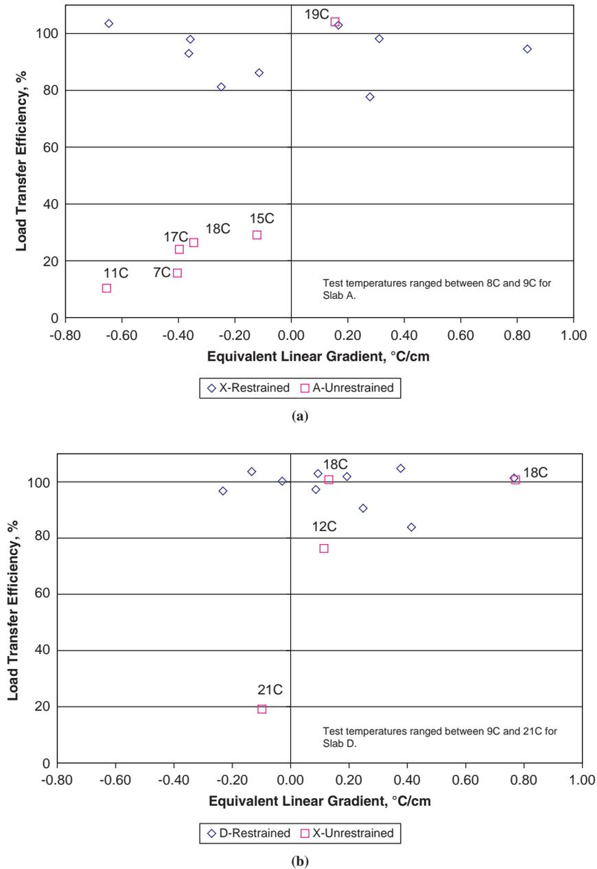
FIGURE 2 Relationship between load transfer and gradients for 190-mm (7.5-in.) slabs on granular base: (a) Cell 5, slab length = 6.1 m (21 ft), and (b) Cell 6, slab length = 4.6 m (15 ft).
