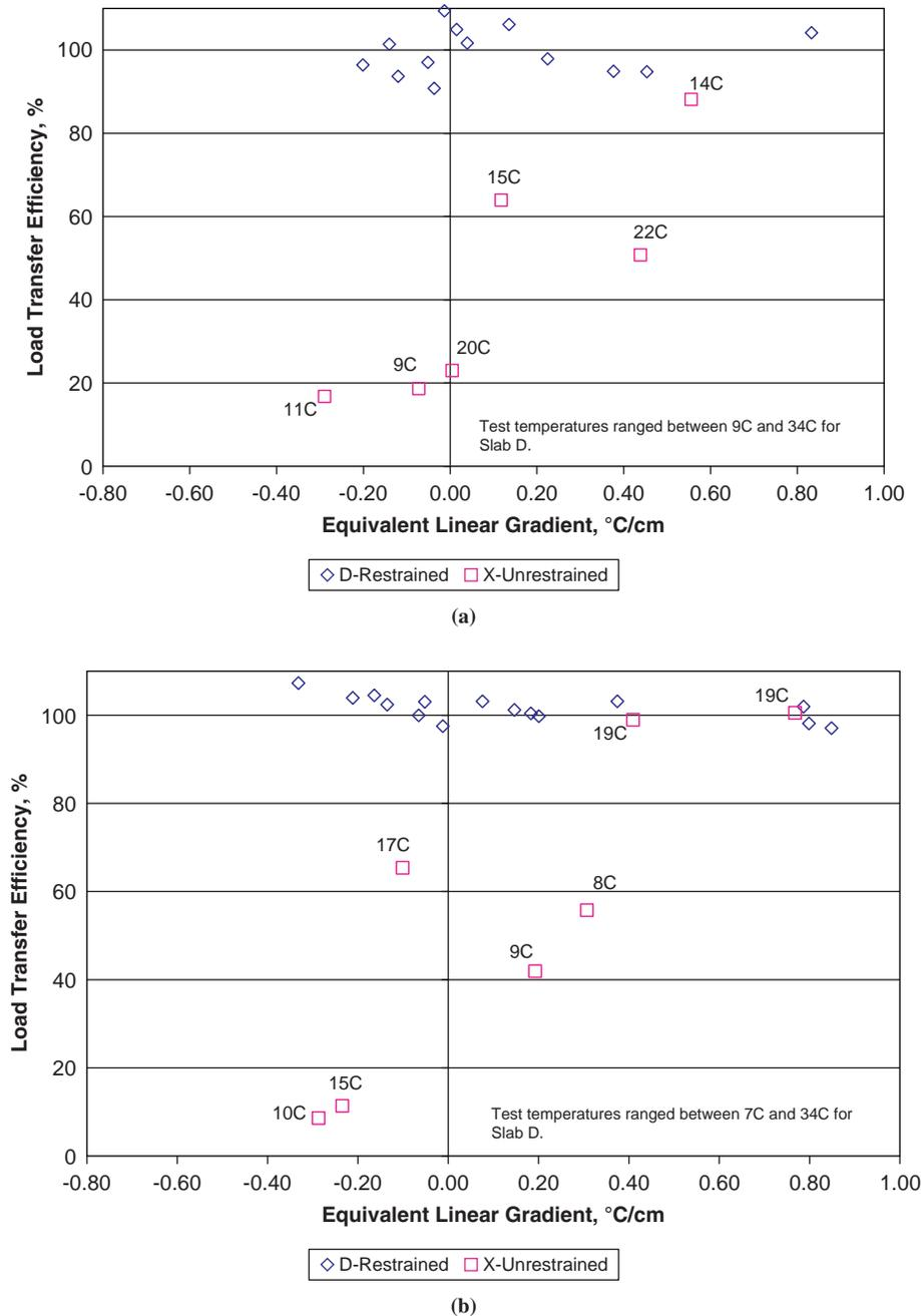
FIGURE 4 Relationship between load transfer and gradients for 240-mm (9.5-in.) slabs with 6.1-m (20-ft) joint spacings: (a) Cell 10, asphalt-stabilized base, and (b) Cell 13, granular base.
