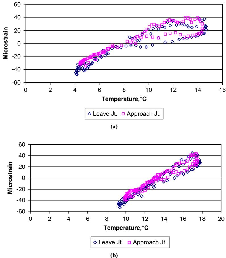
FIGURE 1 Determining occurrence of joint lock-up: (a) strain measurements when joint did lock up and (b) strain measurements when joint did not lock up.
