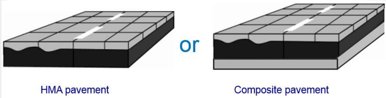
**Figure 1. Pavement types suitable for BCOAs.**
