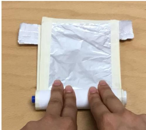
8. After rolling the pieces around the cylinder, secure with masking tape to maintain the shape around the cylinder.
