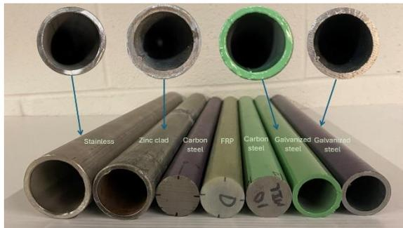
Three replicates per dowel, 21 total specimens
