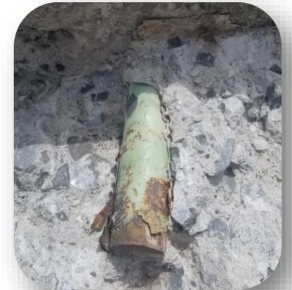
Dowel corrosion model
