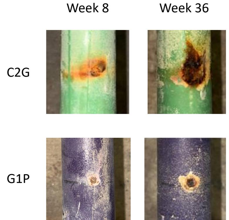
Progressive increase in surface area that corroded was estimated using ImageJ
