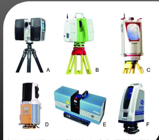
Basic types of terrestrial 3D laser scanners (TLS)-a brief overview. A: Faro Focus 3DX130, B: Leica C10, C: Riegl VZ serie, D: Topcon GLS 1500, E: Surphaser 105HSX, F: Stonex X300.
