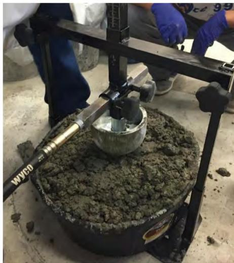
**Figure 12:** Depth of Penetration Under Static Load (National Concrete Pavement Technology Center, 2018)
