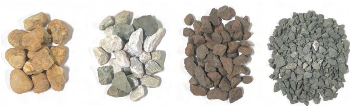
**Figure 17.** Colored aggregates are used to differentiate between particle sizes.
