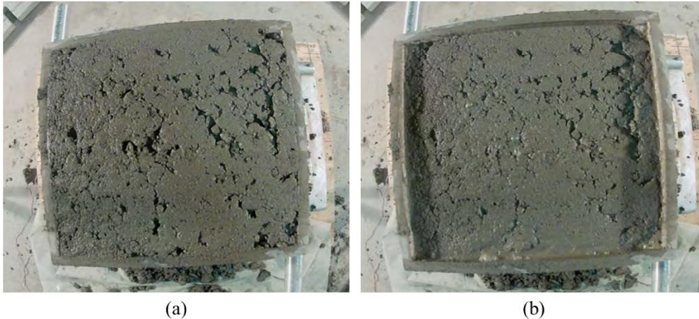
**Figure 18.** Top view of test specimen (a) before and (b) after paving simulation.
