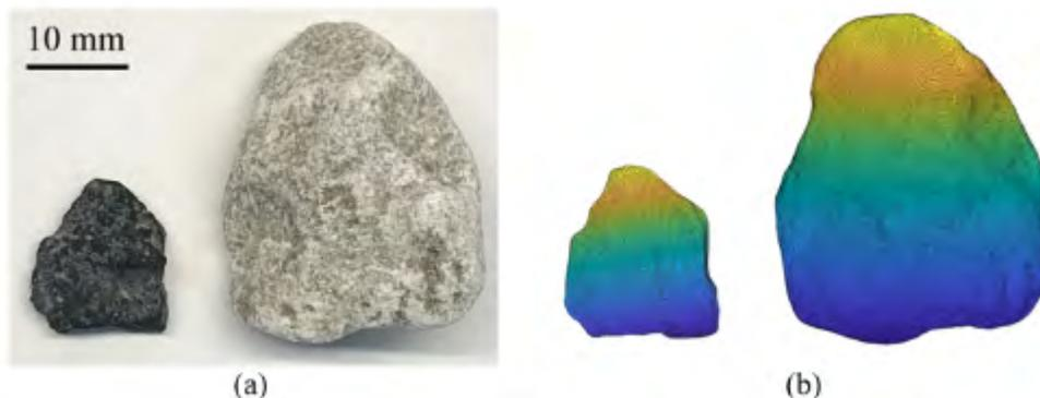
**Figure 28:** Aggregate morphology acquisition, (a) real aggregates (left limestone-01: 0.55 x 0.16 x 0.67 in; right white marble-04: 1.1 x 0.67 x 1.4 in), (b) scanned aggregates (left limestone-01: 6,801 vertices and 13,589 faces; right white marble-04: 30,502 vertices and 61,00 faces).
