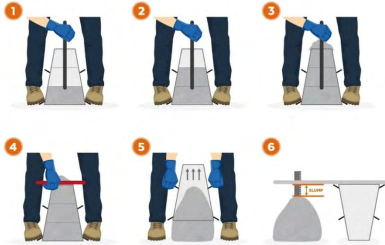
**Figure 9:** Concrete Slump Test (Civil Today, n.d.)
