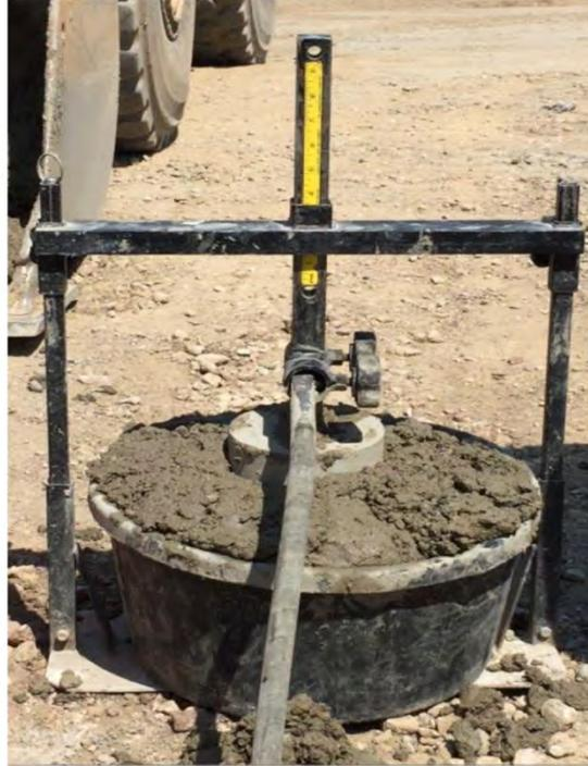
**Figure 13:** Depth of Penetration Under Dynamic Load (National Concrete Pavement Technology Laboratory).
