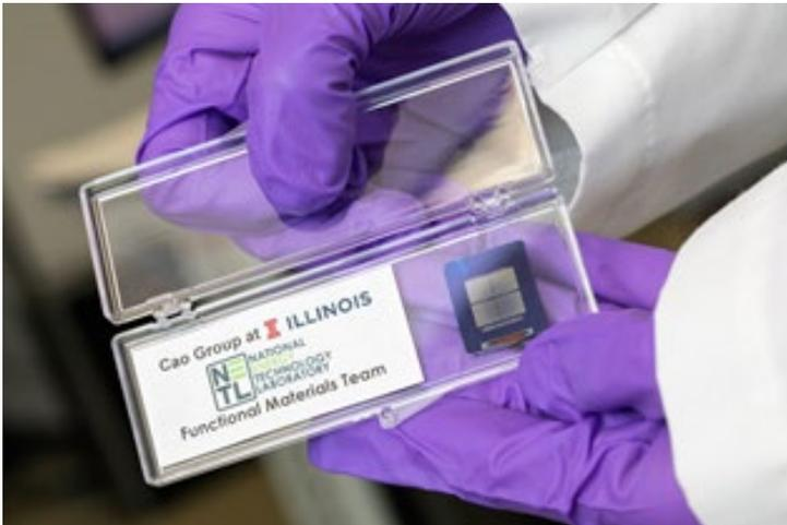
A memristor computer memory device that is enabled by a coal-derived graphene material manufactured at NETL.
