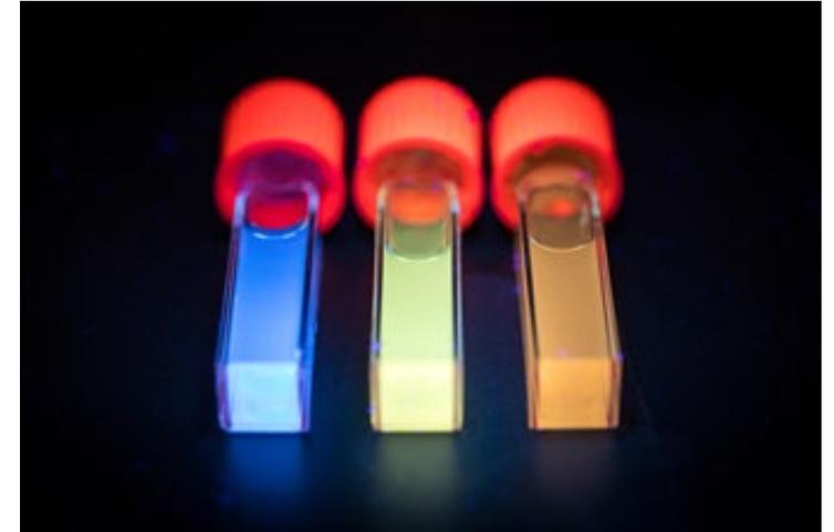
Coal-derived fluorescent graphene quantum dots that are being evaluated for biosensor and medical diagnostic applications.
