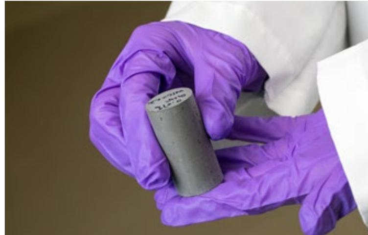
A cement sample that is enhanced with a coal-derived graphene material manufactured at NETL.
