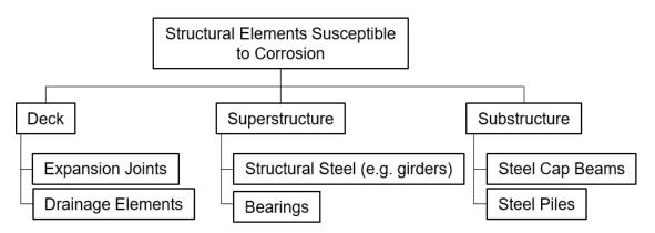
Figure 11. Steel Bridge Components Susceptible to Corrosion (Adapted from [9])
