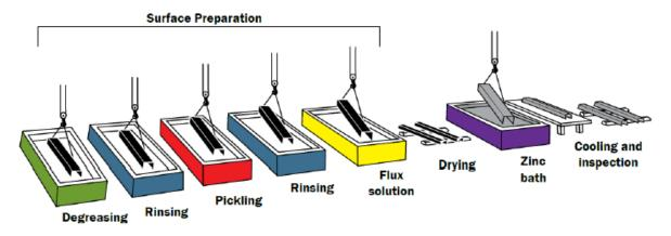
Figure 16. The hot-dip galvanizing process [17]
