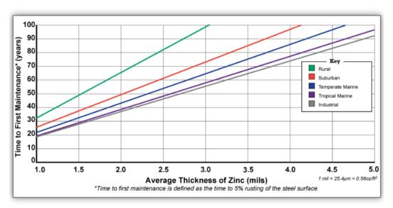
Figure 17 Lifetime prediction of galvanizing steels [19]
