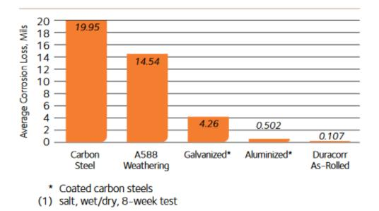
Figure 31 Corrosion Performance in SAEJ2334 Test [50]
