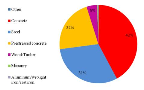
Figure 1 Distribution of Materials Used for Main Spans of US Highway Bridges by Number [3]
