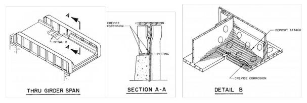
Figure 13. Common Corrosion in Through Girder Span Bridges [6]
