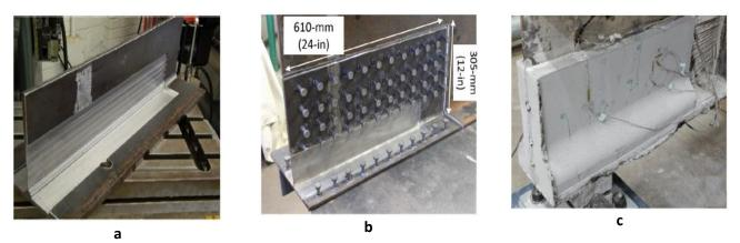
Figure 36 (a) Corrosion simulation on girder; (b) Shear Studs; (c) UHPC Encasement [58]
