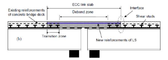
Figure 33 Debonded Link Slab System [54]
