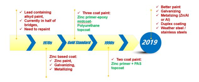
Figure 15. Development of Corrosion-Resistant Coatings for Steel Bridges
