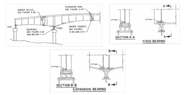
Figure 14. Common Corrosion Patterns in Deck Girder Bridges [6]
