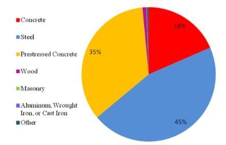
Figure 2. Distribution of Materials Used for Main Spans of US Highway Bridges, by Deck Area
