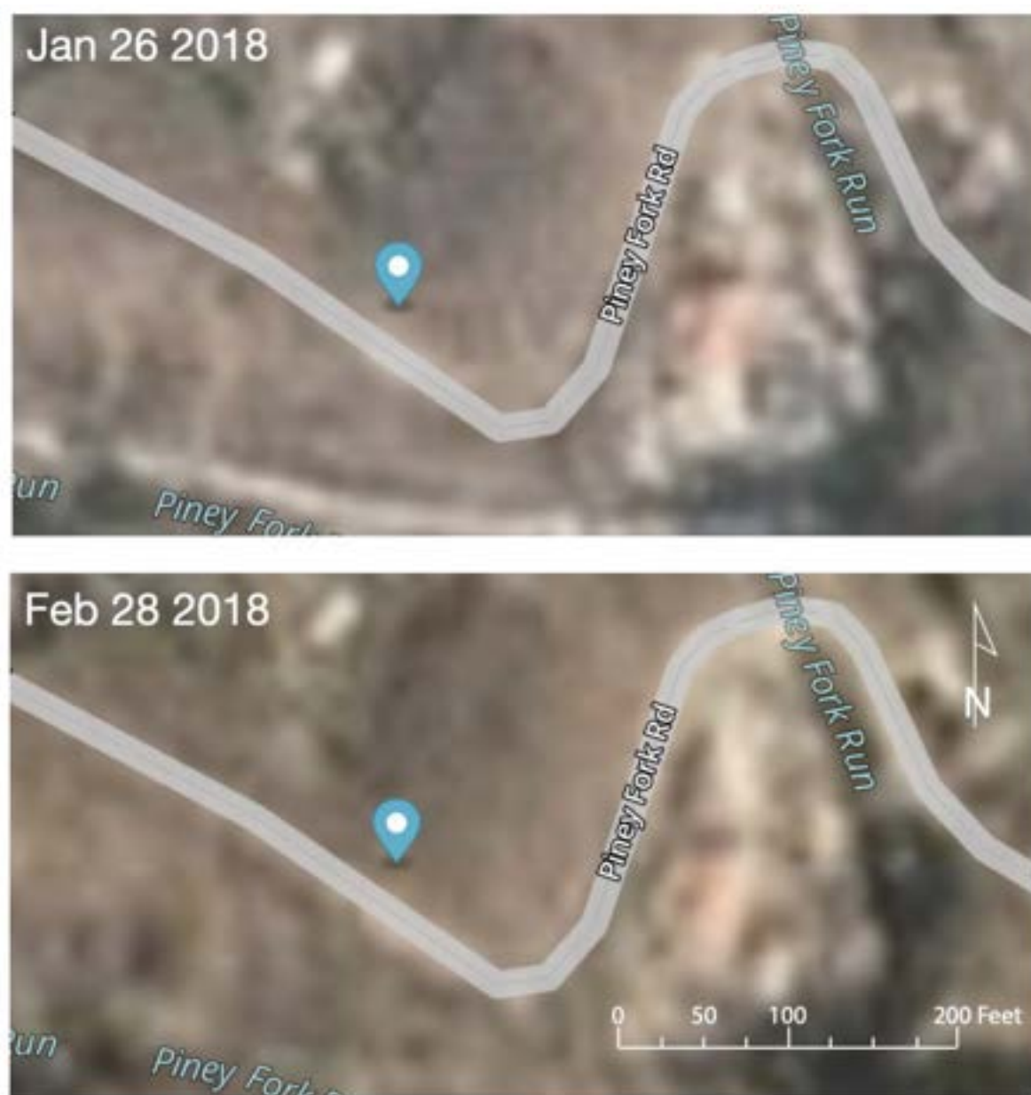
Figure 4.2.3. Return imagery collected by PLANET satellites of a landslide (pin marks approximate location) in Allegheny County reported by PennDOT District 11 on January 29, 2018. Note that change is very hard to detect even at this image of 3m resolution.
