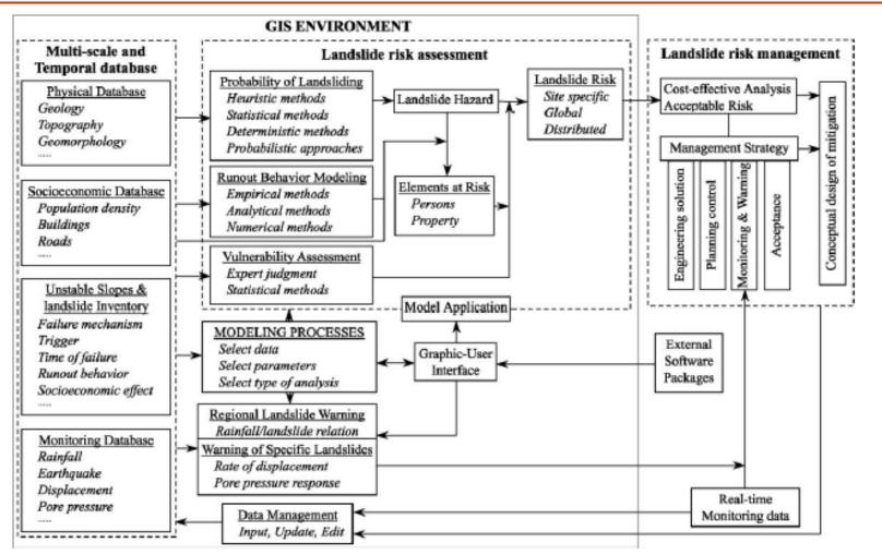
Proposed GIS-based conceptual integrated system for landslide risk assessment and management (Dai et al., *Eng. Geology*, 64, 65-87 <sup>15</sup> University of Pittsburgh
