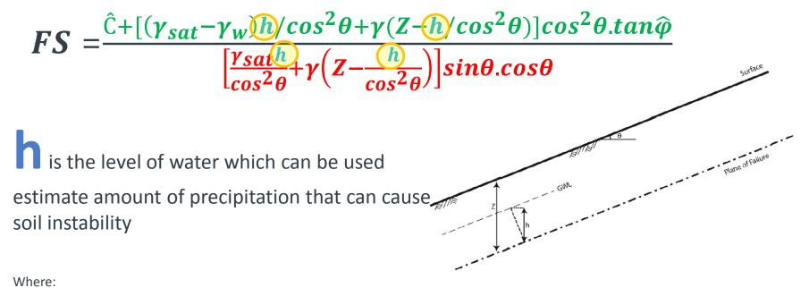
FS= factor of safety H= ground water level  $\gamma_{sat}$  = is the specific weight of saturated soil  $\gamma_w$ =the specific weight of water  $\hat{\varphi}$ =effective internal angle of friction
