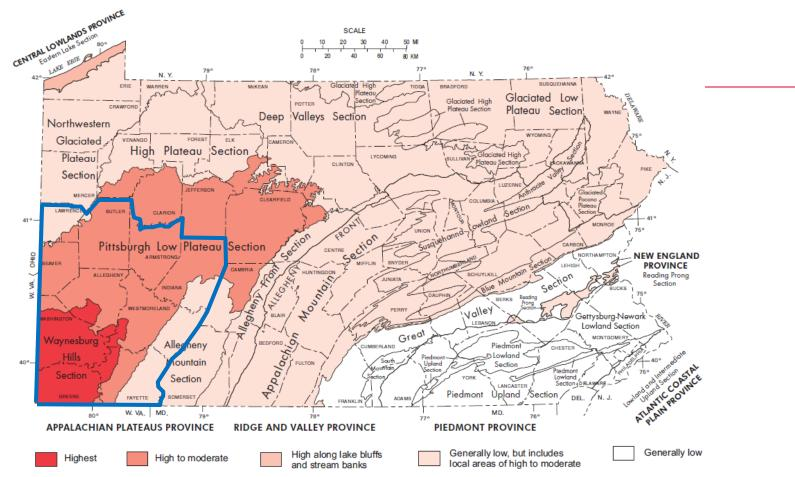
Figure 1. The physiographic provinces and sections of Pennsylvania, and landslide susceptibility.
