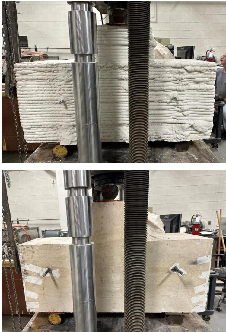
**Figure 17.** Test setup for the prepared 3DCP pier cap
