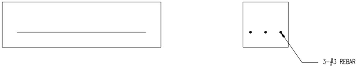
**Figure 4.** Reinforcing details used in the fabricating beam
