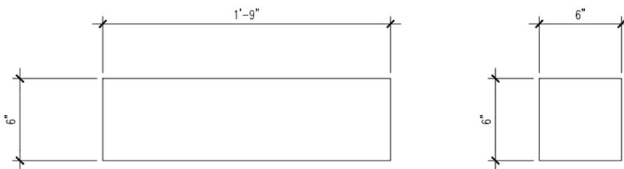
**Figure 3.** Dimensions of the fabricated beam
