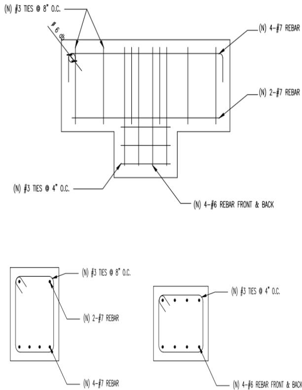
**Figure 12.** Reinforcing detail for pier cap
