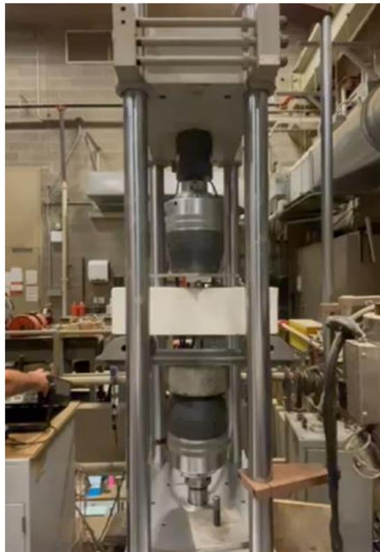
**Figure 7.** Three-point bending test setup
