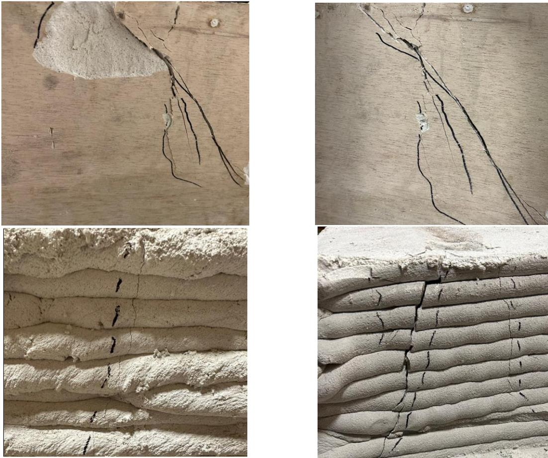
**Figure 18.** Shear failure of pier cap
