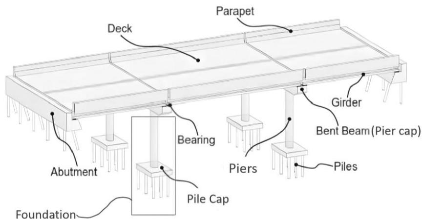
**Figure 10.** Typical bridge components [15]
