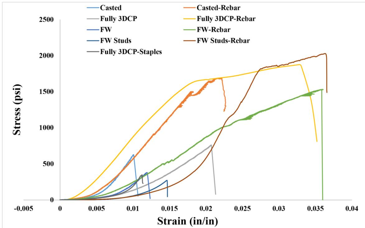
**Figure 9. Strain-stress curve of the fabricated concrete beam**
