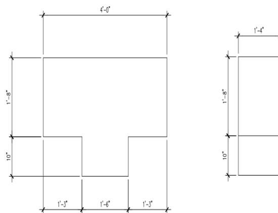
**Figure 11.** Geometry of pier cap (dimensions in inches)
