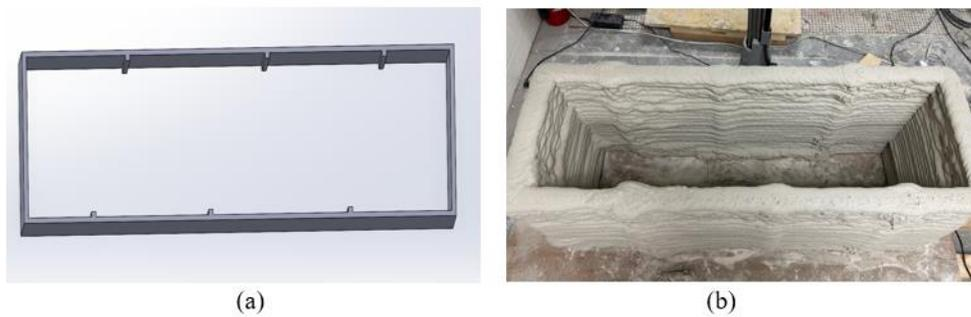
**Figure 15.** (a) Prepared model using SolidWorks and (b) actual printing
