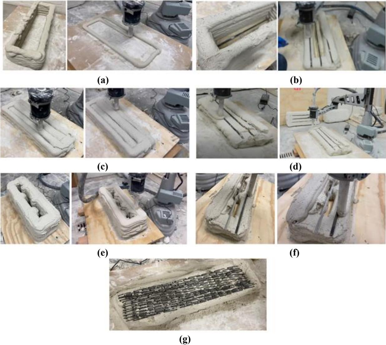
**Figure 6.** Beam fabrication printing process a) plain beam with printed formwork; b) rebar reinforced plain beam with printed formwork; c) plain beam with printed studs formwork; d) rebar reinforced plain beam with printed studs formwork; e) fully printed plain beam; f) fully printed rebar reinforced beam; and g) fully printed staples reinforced beam
