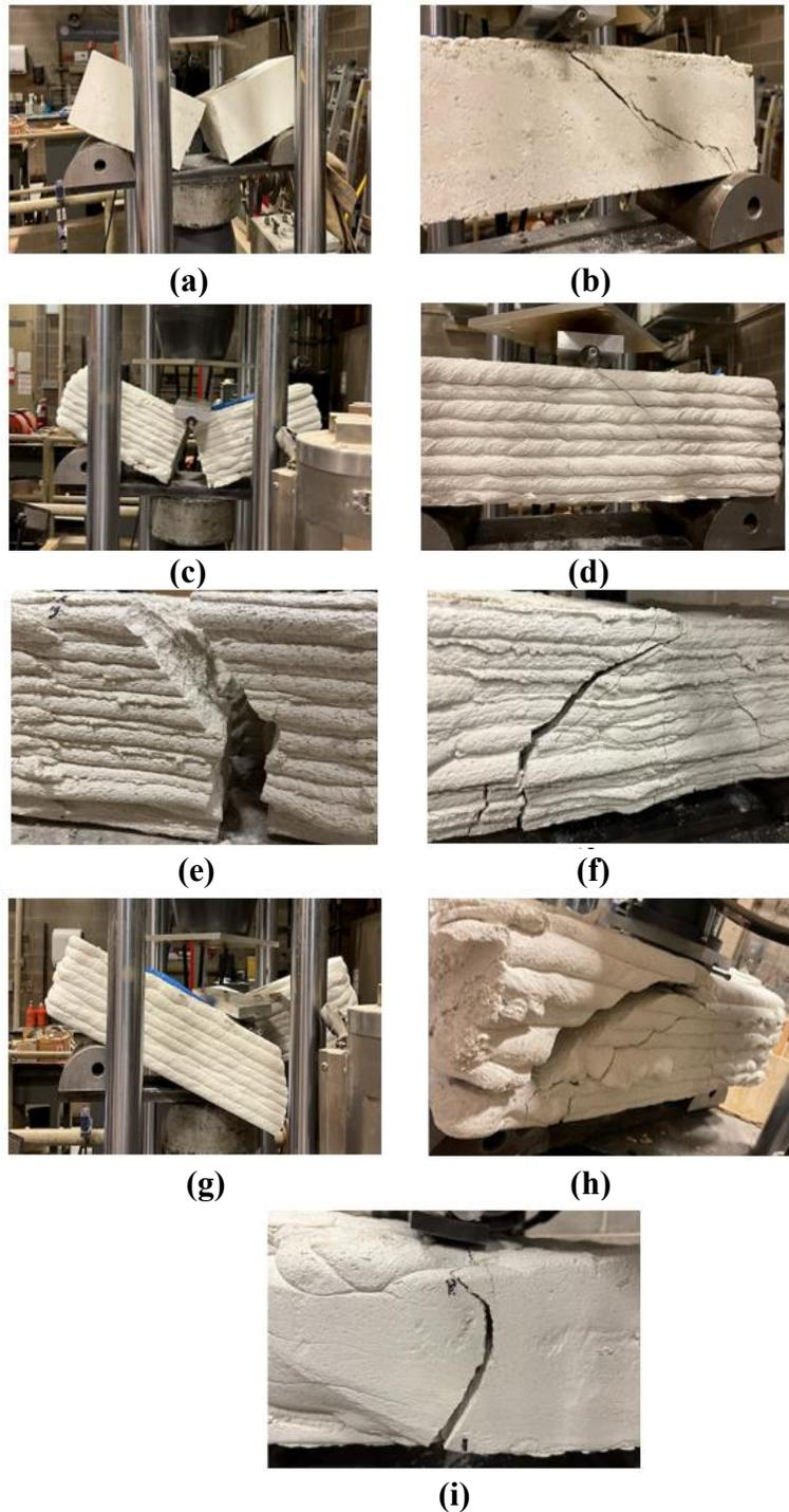
**Figure 8.** Failure Beams a) Cast plain beam; b) cast rebar reinforced beam; c) plain beam with printed formwork; d) rebar reinforced plain beam with printed formwork; e) plain beam with printed studs formwork; f) rebar reinforced plain beam with printed studs formwork; g) fully printed plain beam; h) fully printed rebar reinforced beam; i) fully printed staples reinforced beam
