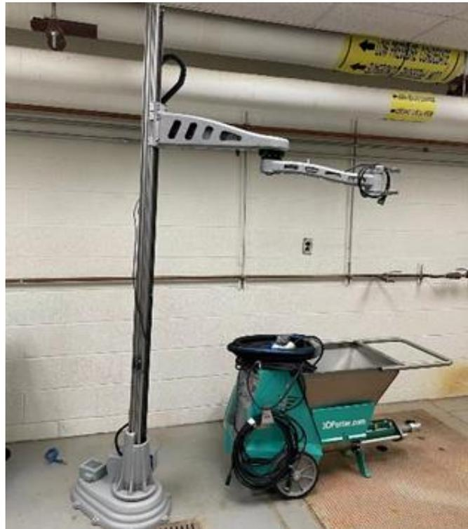
**Figure 2.** 3D concrete printing machine and pump used in this project
