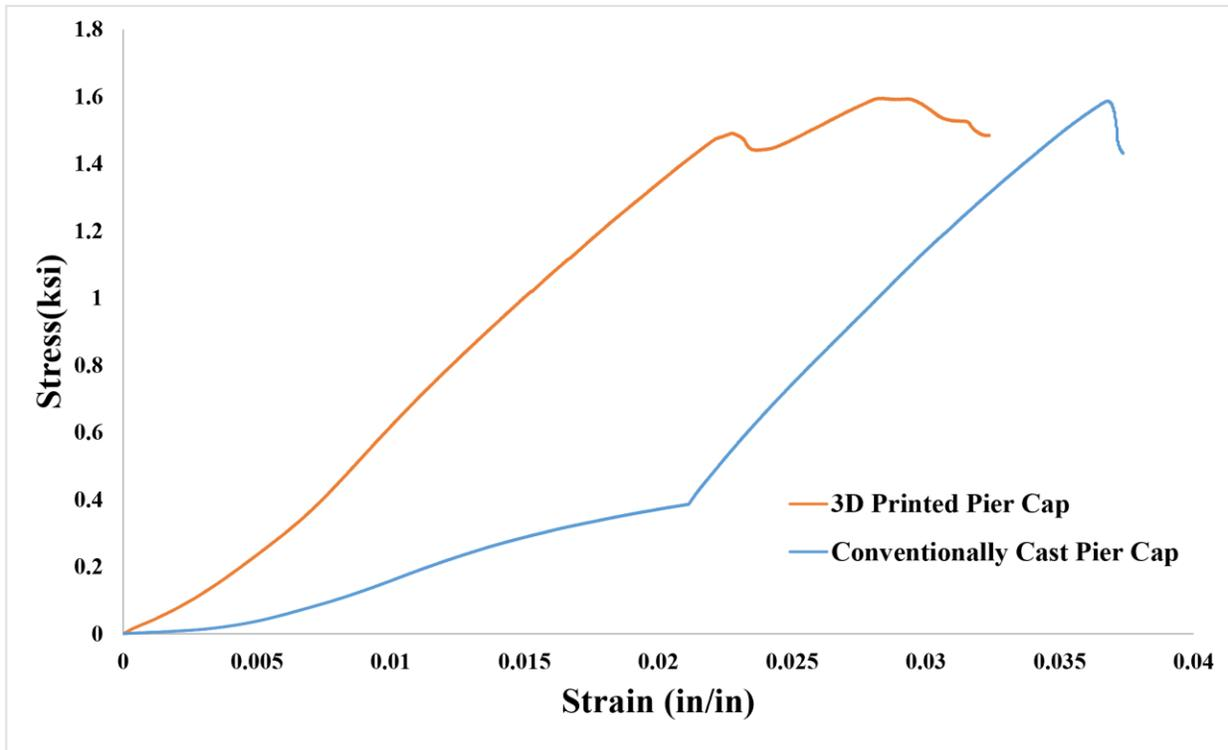
Figure 19. Stress-strain curve obtained during compression test
