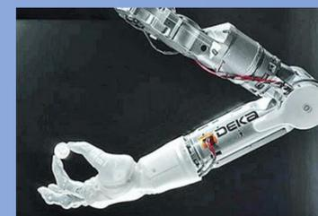
The DEKA "Luke Arm" produced by Mobius Bionics and is capable of higher motor function.
