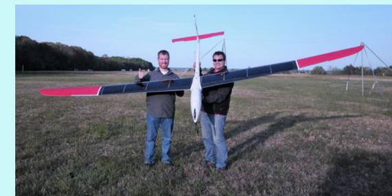
Image showing the modified SBXC sailplane constructed by the Naval Research Laboratory
