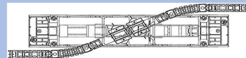
"S" shaped conveyer design (underneath machine)
