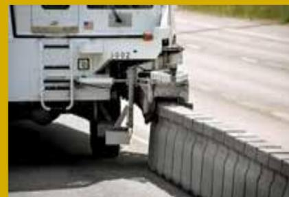
1. One- meter sections of highly reinforced concrete barriers are pinned together at each end to form a continuous wall. The barriers are designed with a "T" shaped top used as the lifting surface for the barrier.
