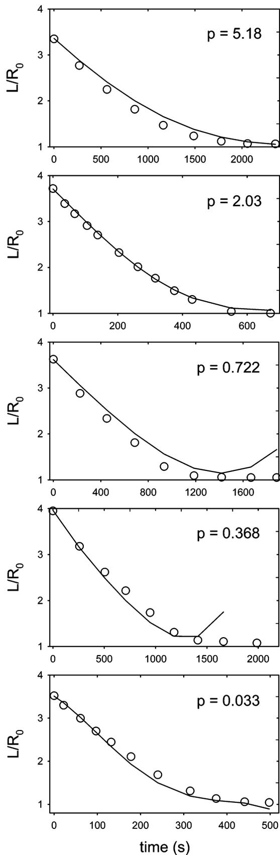
**Figure 3.** Fiber retraction results plotted in the form required by the TOS model. Solid lines are eq 5 with  $\sigma$  being the equilibrium interfacial tension  $\sigma_{eq}$  listed in Table 2. The upturns in the solid lines at  $p = 0.368$  and  $0.722$  are artifacts of the fourth-order polynomial approximation of the TOS model.
