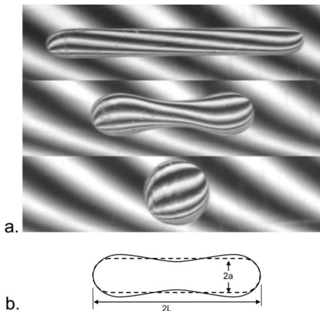
**Figure 1.** (a) Shapes of a drop with  $p = 0.368$  during retraction. The alternating black and white stripe pattern in the background helps define the edge of the fiber clearly even if the refractive index difference of the fiber is close to that of the matrix. (b) Geometric parameters for analysis: The dotted line a spherocylinder of the same length and volume as the actual drop. The diameter  $2a$  is obtained by solving eq 1.
