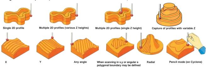
Stage 2 - Data Manipulation Tracecut can be used to easily manipulate the captured data for multiple practical applications -
