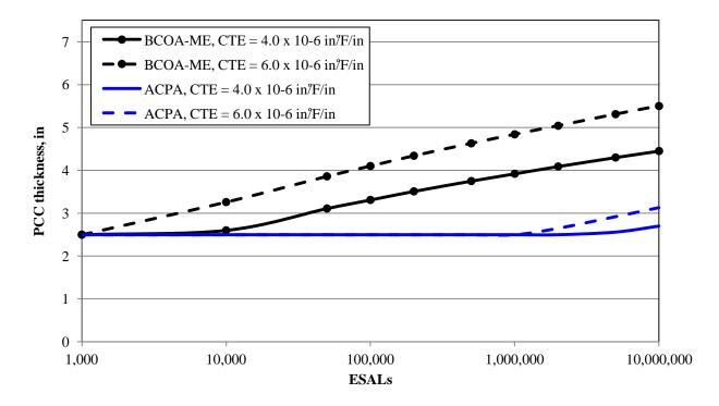
Figure 6. PCC thickness sensitivity to coefficient of thermal expansion for 4 ft  $\times$  4 ft slabs with respect to design ESALs
