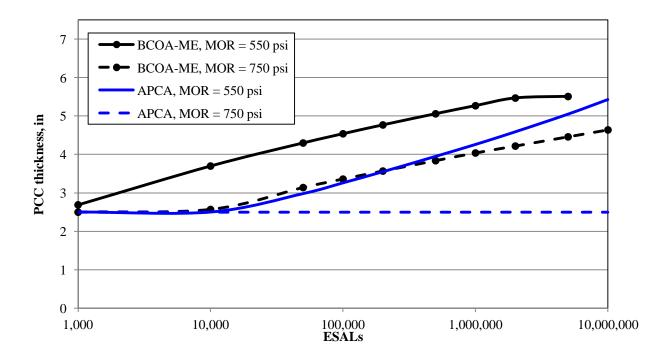
Figure 3. PCC thickness sensitivity to PCC modulus of rupture for 4 ft  $\times$  4 ft slabs with respect to design ESALs
