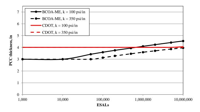
Figure 16. PCC thickness sensitivity to k value for 6 ft  $\times$  6 ft slabs with respect to design ESALs
