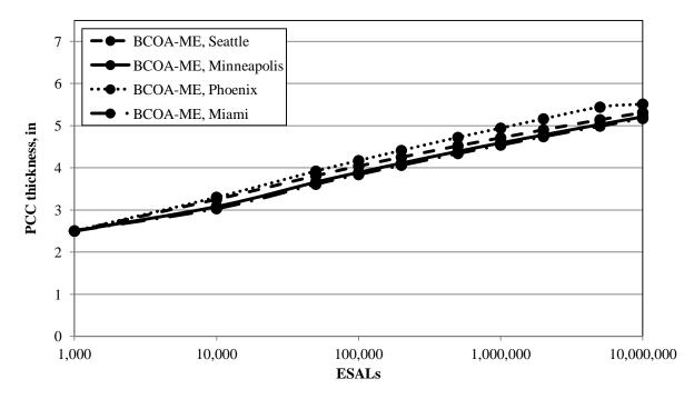
Figure 18. PCC thickness sensitivity to climate for 4 ft  $\times$  4 ft slabs with respect to design ESALs
