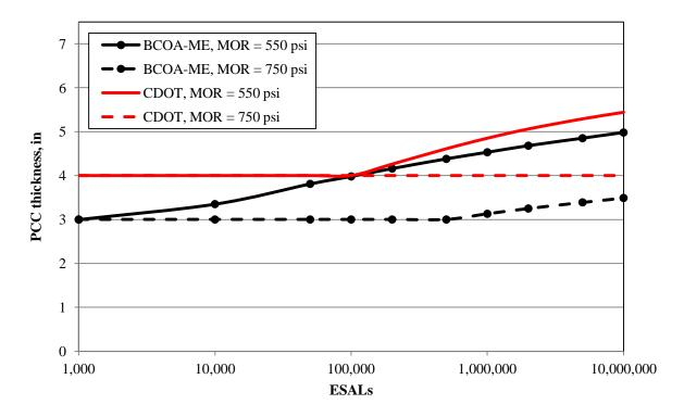
Figure 4. PCC thickness sensitivity to PCC modulus of rupture for 6 ft  $\times$  6 ft slabs with respect to design ESALs
