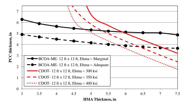
Figure 14. PCC thickness sensitivity to HMA quality for 12 ft  $\times$  12 ft slabs with respect to HMA thickness
