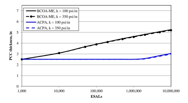
Figure 15. PCC thickness sensitivity to k value for 4 ft  $\times$  4 ft slabs with respect to design ESALs
