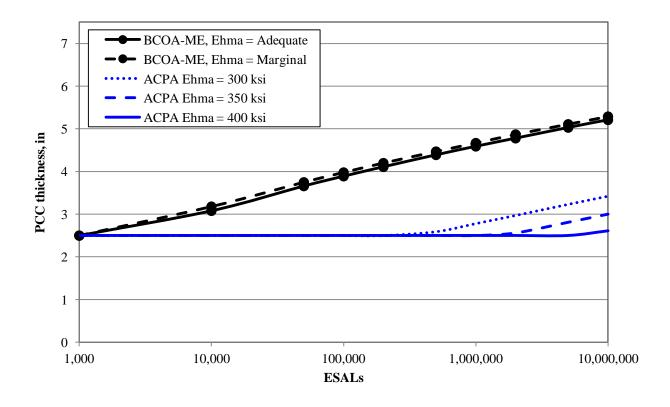
Figure 9. PCC thickness sensitivity to HMA quality for 4 ft  $\times$  4 ft slabs with respect to design ESALs
