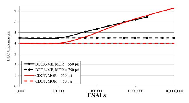
Figure 5. PCC thickness sensitivity to PCC modulus of rupture for  $12 \text{ ft} \times 12 \text{ ft}$  slabs with respect to design ESALs
