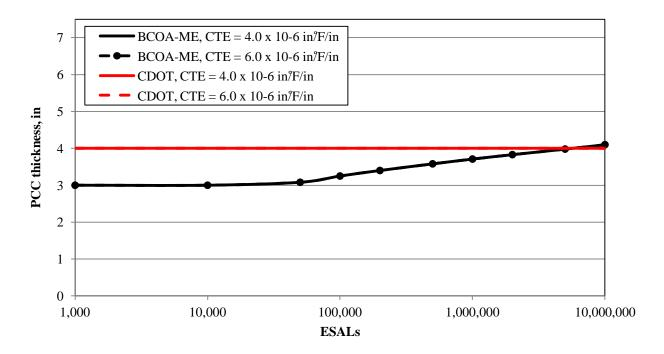
Figure 7. PCC thickness sensitivity to coefficient of thermal expansion for 6 ft  $\times$  6 ft slabs with respect to design ESALs
