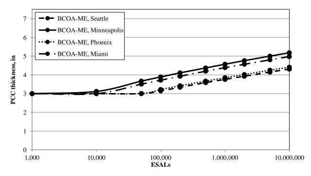
Figure 20. PCC thickness sensitivity to climate for 12 ft  $\times$  12 ft slabs with respect to design ESALs
