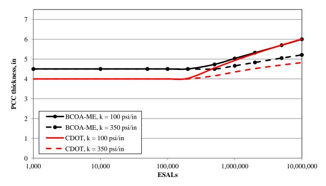
Figure 17. PCC thickness sensitivity to k value for 12 ft  $\times$  12 ft slabs with respect to design ESALs
