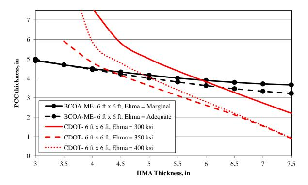
Figure 12. PCC thickness sensitivity to HMA quality for 6 ft  $\times$  6 ft slabs with respect to HMA thickness
