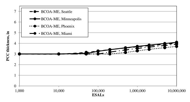
Figure 19. PCC thickness sensitivity to climate for 6 ft  $\times$  6 ft slabs with respect to design ESALs
