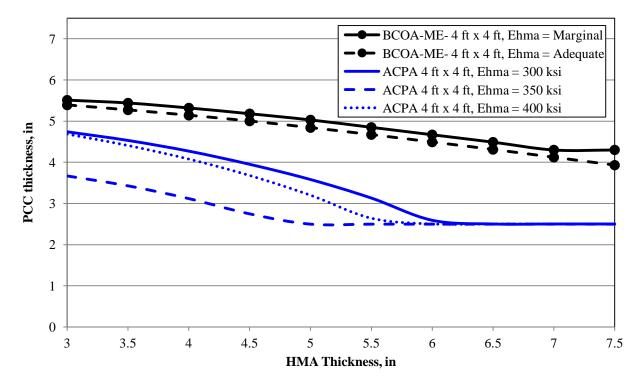
Figure 10. PCC thickness sensitivity to HMA quality for 4 ft  $\times$  4 ft slabs with respect to HMA thickness
