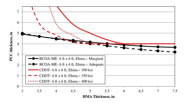
Figure 11. PCC thickness sensitivity to HMA quality for 6 ft  $\times$  6 ft slabs with respect to HMA thickness
