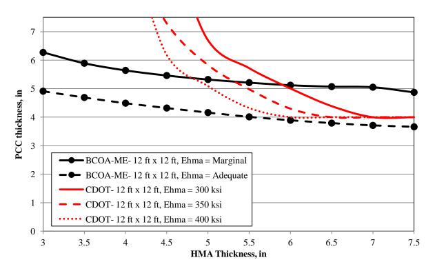
Figure 13. PCC thickness sensitivity to HMA quality for 12 ft  $\times$  12 ft slabs with respect to HMA thickness
