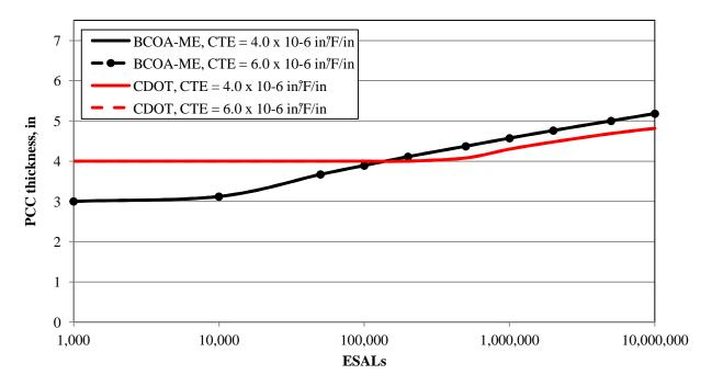
Figure 8. PCC thickness sensitivity to coefficient of thermal expansion for  $12 \text{ ft} \times 12 \text{ ft}$  slabs with respect to design ESALs
